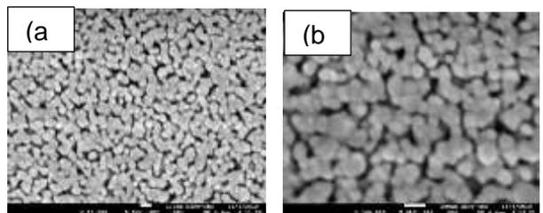
Figure 6: TiO<sub>2</sub>/ZnO bilayer thin films annealed at 600°C for magnification (a) 50,000 and (b) 100,000x [4]
