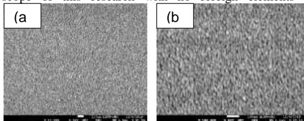
Figure 4: TiO<sub>2</sub>/ZnO bilayer thin films annealed at 400°C for magnification (a) 50,000 and (b) 100,000x
