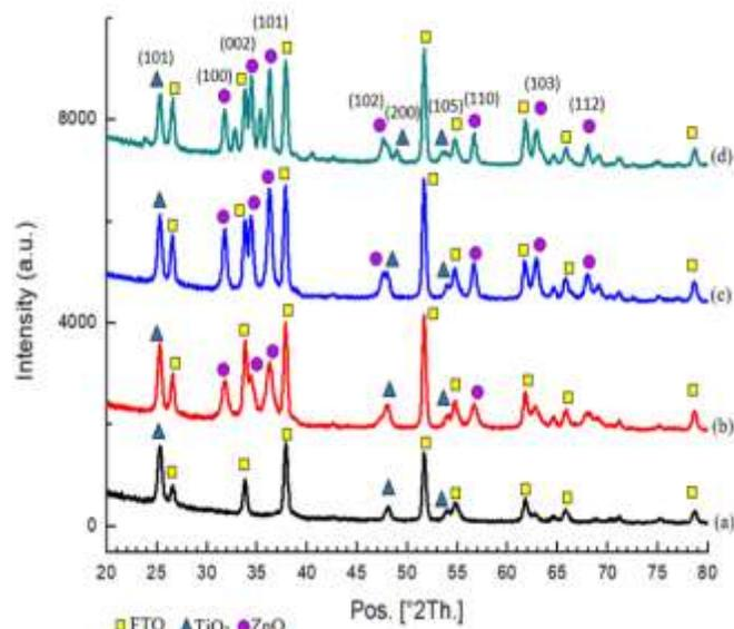
TiO<sub>2</sub>/ZnO bilayer thin film to get better structural properties. This is because the peak intensity is the highest with no foreign elements or compound were present.
