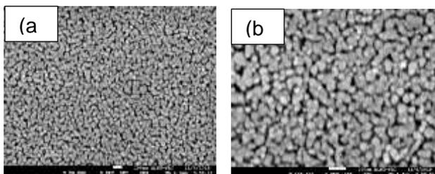
Figure 5: TiO<sub>2</sub>/ZnO bilayer thin films annealed at 500°C for magnification (a) 50,000 and (b) 100,000x
