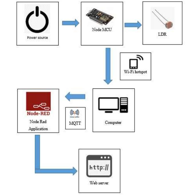
Figure 2. Block diagram for smart streetlight system
