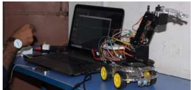
Figure 6: Operator controlling the robot arm using right hand
