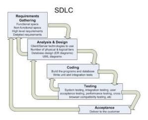
**Figure 1.** Waterfall Model of System Development Life Cycle (SDLC).
