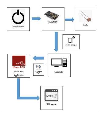
Figure 2. Block diagram for smart streetlight system
