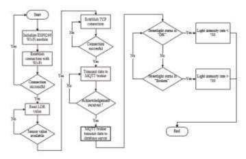
Figure 1. Flowchart for smart streetlight system
