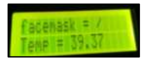
Figure 4. The LCD display shows a visitor's temperature higher than 37.5°C and do not wear or wearing an imperfect face mask.
