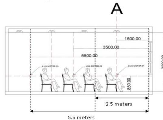
Figure 5. Experimental set-up on the writing performance
